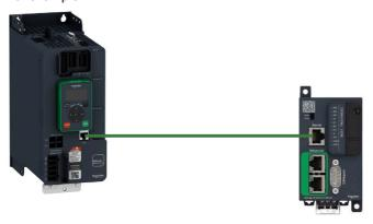
The drive is controlled from the communication (Modbus serial) but the reference value is adjusted with analog input 1. The control word comes from the controller and is written according to CiA 402 profile.
